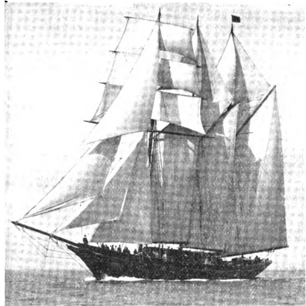
La Cigale. R. Y. S. Lt. Col. A. M. B. Gage, Owner. Designed by C. E. Nicholson. Built by Camper & Nicholson. Length O. A. 122.2 Ft., L. W. L. 100 Ft., Breadth 23.72 Ft., Draught 13 Ft. 295 Tons. Power Two Parsons Paraffin Engines 65-H.P. Each. Speed in Dead Calm 8 Knots
